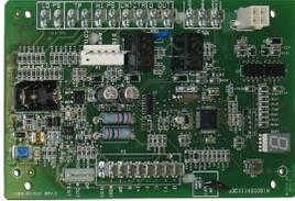
Auto Configuration - On start-up the control automatically sends a description of the unit to the iComfort® Communicating Thermostat to automatically configure the features available.
